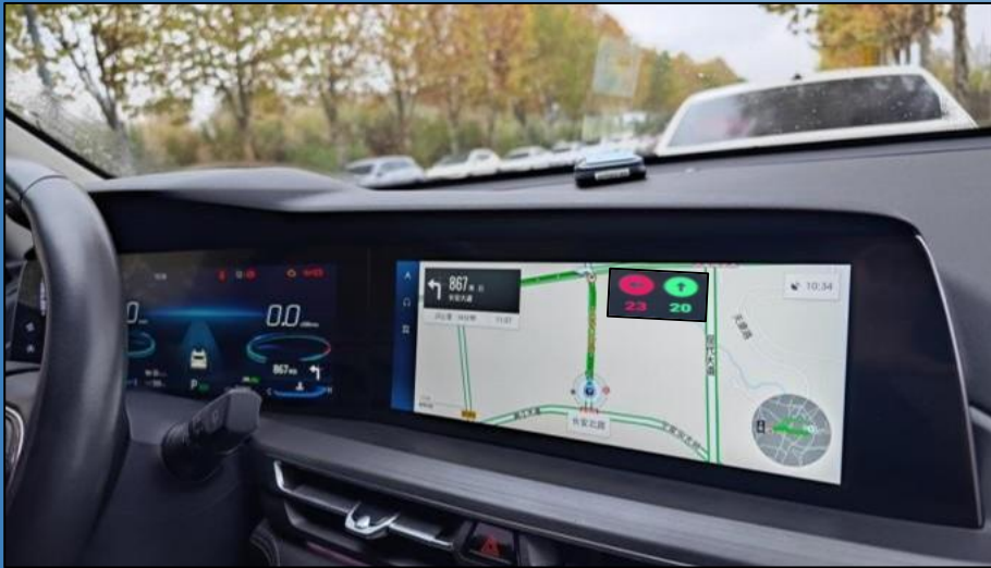
基于Uu的网联预警提醒功能 Uu-based networking warning alert function
